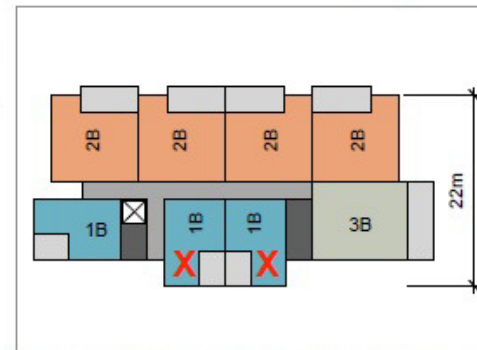
Melbourne / Victoria compliant plan has only 1 core with lower cross ventilation requirements
