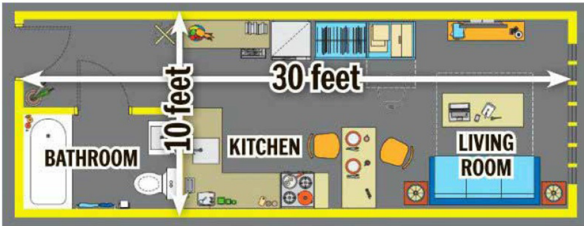
A 300 square feet or 30 square metre micro unit design for Mayor Bloomberg's competition
